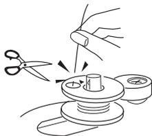
5 With the free end of the thread held in your hand, start the machine. Stop the machine when it has wound a few layers, and then cut the thread close to the hole in the bobbin.
