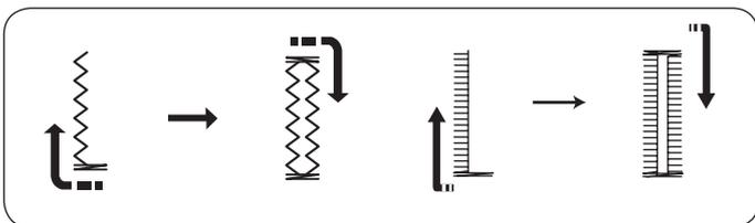
The machine will sew the front bartack and left row first. The machine will sew the back bartack and right row, then it stops automatically. The stitch width can be varied from 2.5 to 7.0. The stitch density can be varied from 0.5 to 1.0 (Stretch buttonhole), 0.5 to 2.5 (Antique buttonhole).
