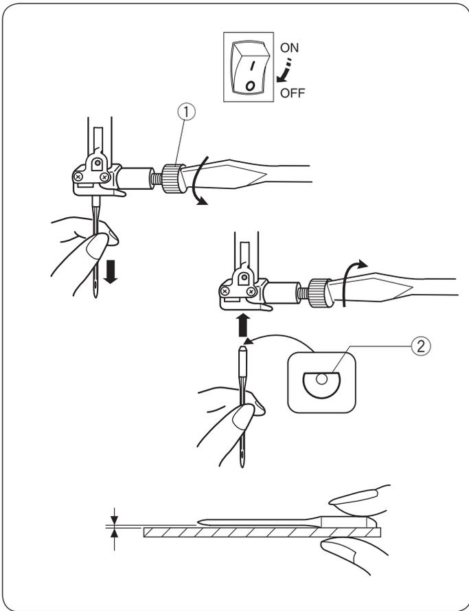
Loosen the needle clamp screw by turning it counterclockwise with a screwdriver. Remove the needle from the needle clamp.
