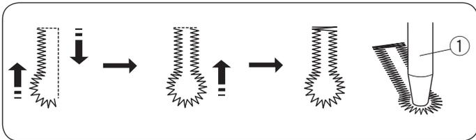
Sewing procedure is the same as square buttonhole. The buttonhole width can be varied from 5.5 to 7.0. The stitch density can be varied from 0.3 to 0.8. Use the seam ripper and an eyelet punch to open the buttonhole.
