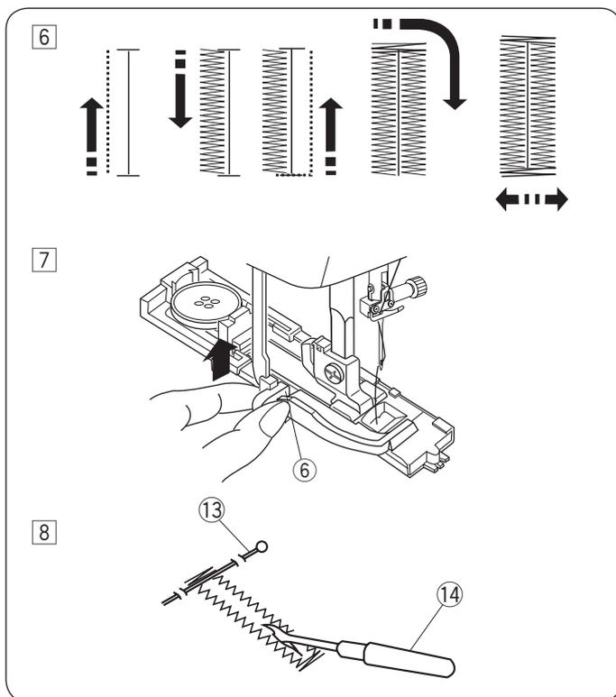
6 The buttonhole is sewn in the sequence as shown. When the buttonhole is finished, the machine will stop automatically with the needle in the up position.
