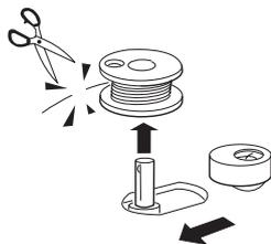
6 Start the machine. When the bobbin is fully wound, it will stop spinning automatically.
