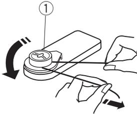
1 Draw the thread from the spool and pass the thread around the bobbin winding tension disk.
