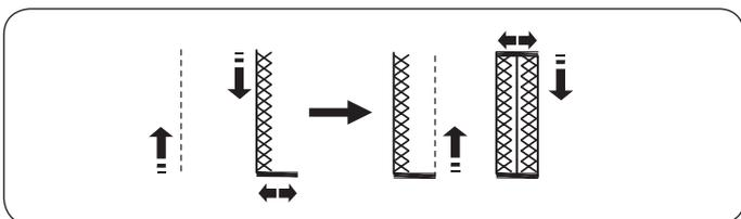
Sewing procedure is the same as square buttonhole. The buttonhole width can be varied from 2.5 to 7.0. The stitch density can be varied from 0.7 to 1.2.
