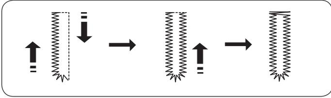
Sewing procedure is the same as square buttonhole. The buttonhole width can be varied from 2.5 to 5.5. The stitch density can be varied from 0.2 to 0.8.
